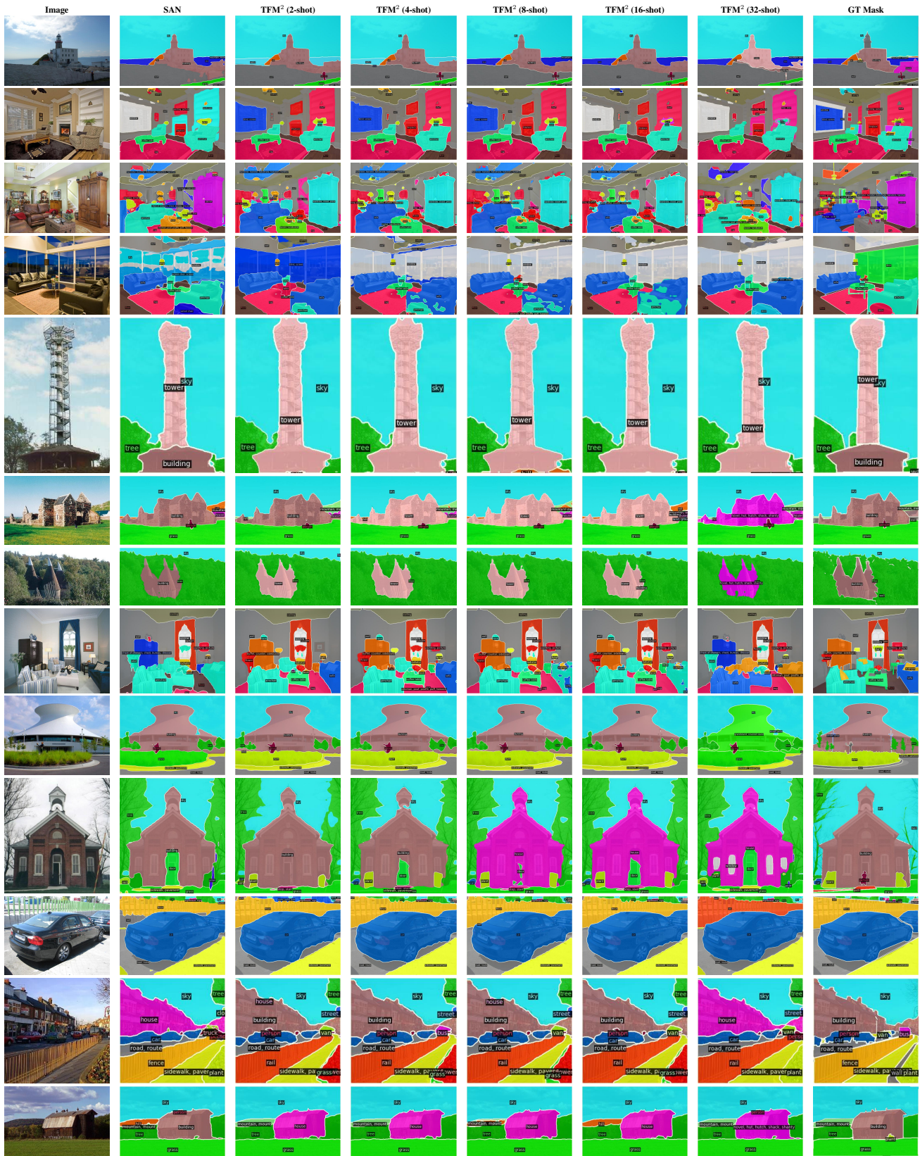
Figure 3. Qualitative examples showing TFM 2 sometimes can not improve mask proposal classification on ADE20k-150. The second column shows SAN inference without TFM 2 . We see that SAN + TFM 2 (third column to seventh column) sometimes misclassified some mask proposals (compared with the ground truth in the last column). Please note that the color palette is the same for all mask classes.
